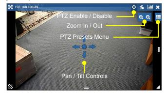
**To control PTZ:** Enable PTZ control by clicking on the **PTZ** icon. Then use the Pan/Tilt controls and the Zoom controls that appear on-screen. (Control is available using a mouse, joystick, or touch supported inputs.) Use the *Presets Menu* to switch between predefined camera views.
