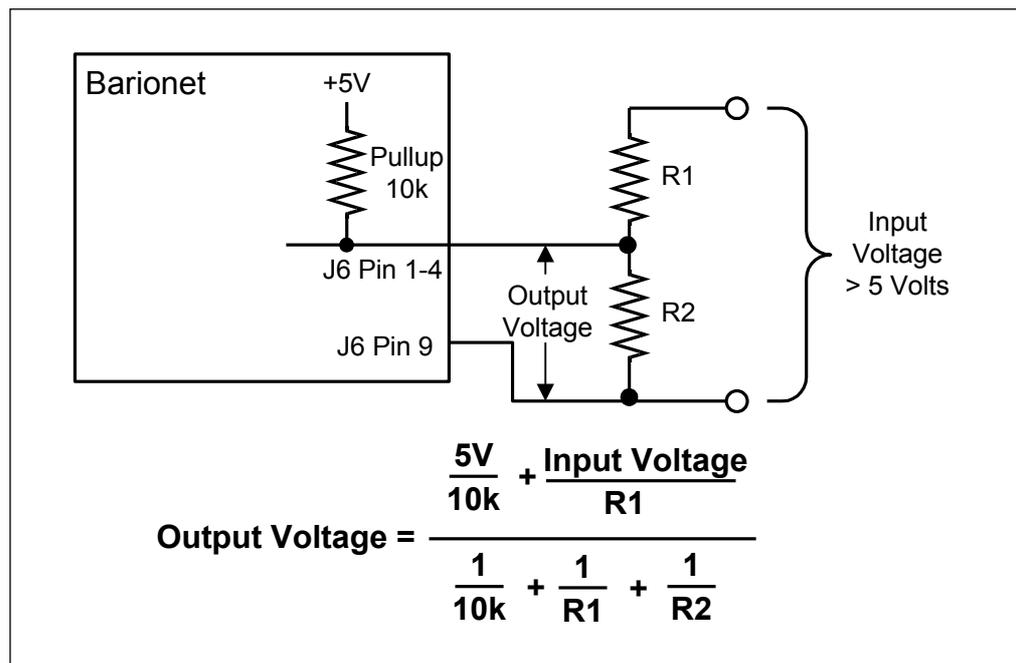
Figure 24. The effects of turning on the 10kΩ pull-up resistor on the voltage divider.
