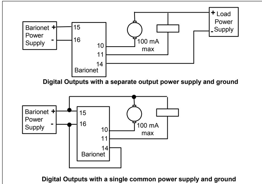
Figure 27. Digital outputs can use a separate power supply and ground or a common power supply and ground.
