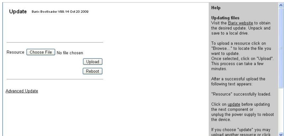
Figure 41. When the Barionet 50 restarts in Boot Loader mode, this Update screen appears.
