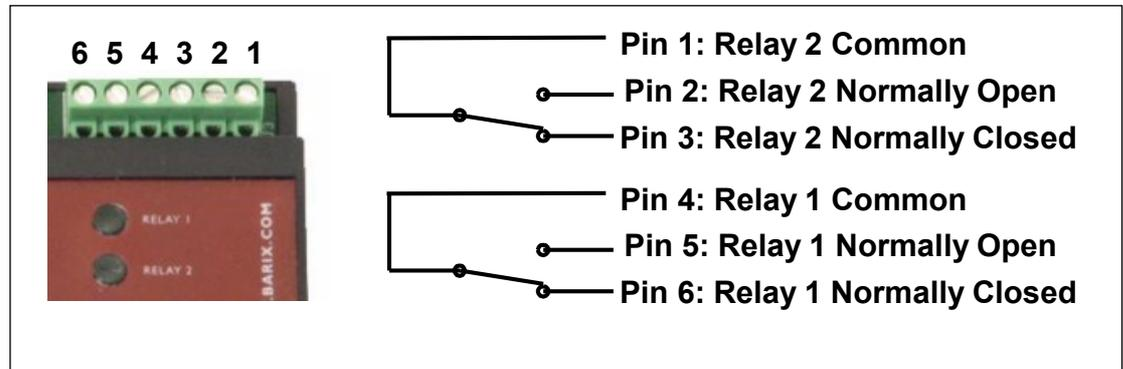
Figure 22. The Barionet Relay Outputs.
