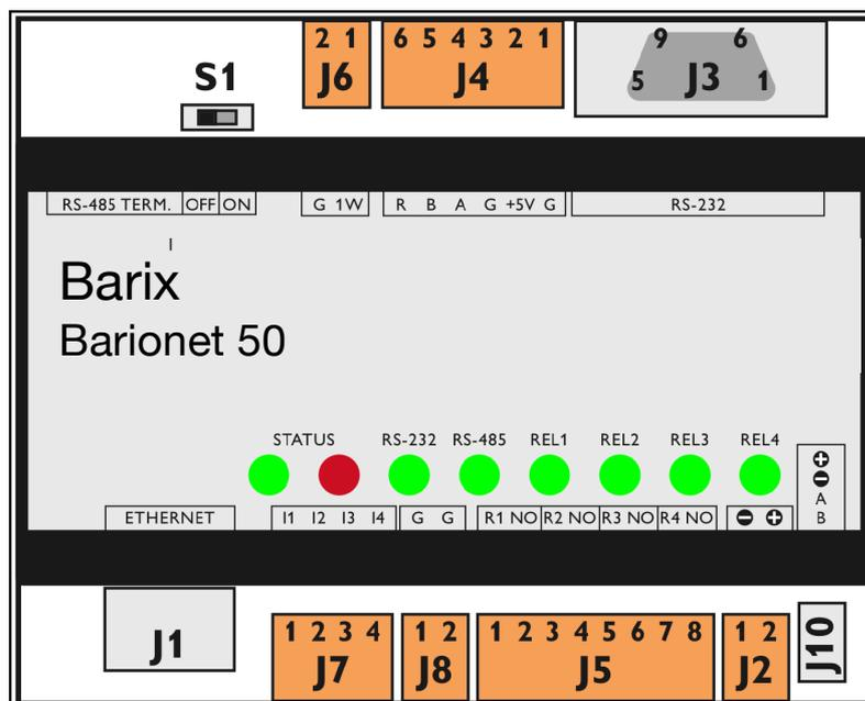
Figure 28. The Barionet 50 connectors and indicators.
